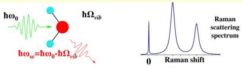
Raman spectrum reflects the vibrational spectrum of material and provides the information about its chemical content and phase state.
