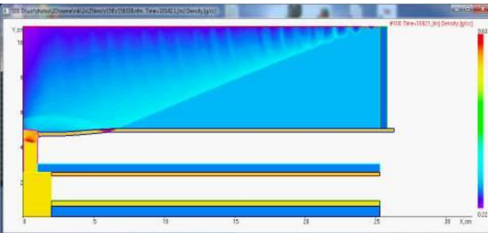
10020 ns. Launching of 1-st stage liner. Cone formation
