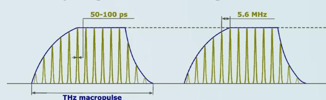
Schematic view of NovoFEL radiation macropulses. The length of the individual THz pulse and their repetition rate are shown for the first FEL.
