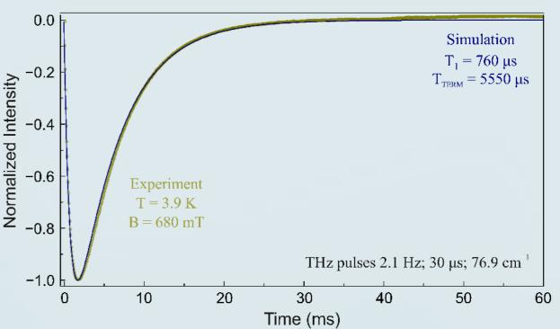
Least square fitting of the experimental data obtained by T-jump spectroscopy by the proposed numerical model.
