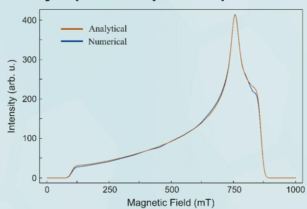
Comparison of the calculated EPR signal induced by T-jump and analytical calculation of the lineshape for the model system with effective spin 1/2. The numerical simulation was performed for 400,000 random orientations. The inhomogeneous linewidth was 10 mT. The spectrometer frequency was 9.75 GHz.
