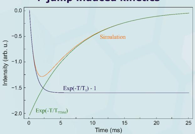
Comparison of the kinetics traces obtained from the numerical simulation (orange) with exponential thermal relaxation with a characteristic time of 7 ms ( $\exp(-T/T_{TERM})$ , green) and exponential  $T_1$  relaxation with a characteristic time of 750 µs (exp(-T/ $T_1$ ) - 1, dark blue).
