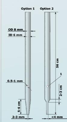
THz radiation is transmitted to the sample using a special hollow metal/dielectric waveguide. The transmission coefficient of the waveguides is about 0.65 (4.4 dB/m) at 45.5 cm<sup>-1</sup>. THz radiation with a wavenumber of 76.9 cm<sup>-1</sup> was used in the experiments. To ensure maximum sensitivity to  $T_1$  of the sample, the macropulse duration was 30 μs at 4.5 Hz repetition rate.
