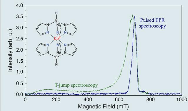
Comparison of spectra of bis[tris(pyrazolyl)borate] cobalt(II) with 1% concentration of paramagnetic ions at 4.2 K.
