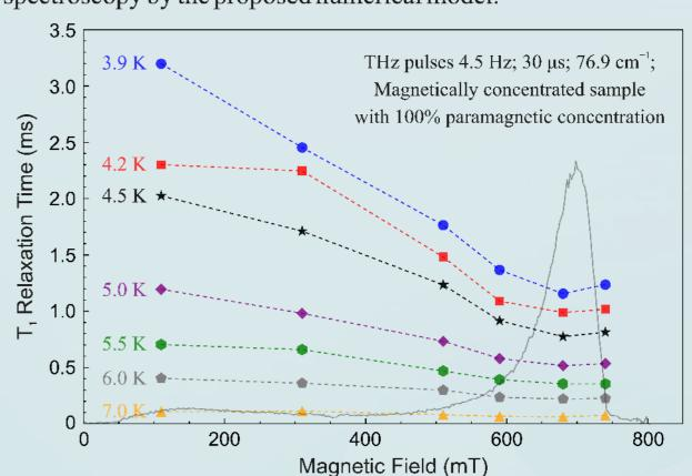
Orientation and temperature dependencies of T<sub>1</sub> relaxation time of bis[tris(pyrazolyl)borate] cobalt(II) measured by T-jump spectroscopy under pulsed heating by THz irradiation.
