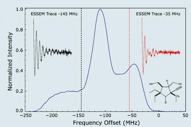
Phase corrected FT spectrum of nitroxide obtained using WURST pulses and its ESEEM traces at -145 and -35 MHz offsets.
