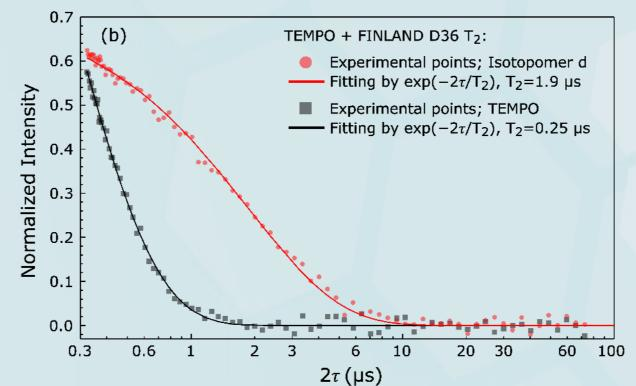
Two pulse echo measurements of 30 µM TEMPO and 10 µM Finland trityl D36. (a) Phase corrected FT spectrum at 170 ns; (b) echo decay for the high field TEMPO line and for the high field line of the trityl isotopomer 'd'.
