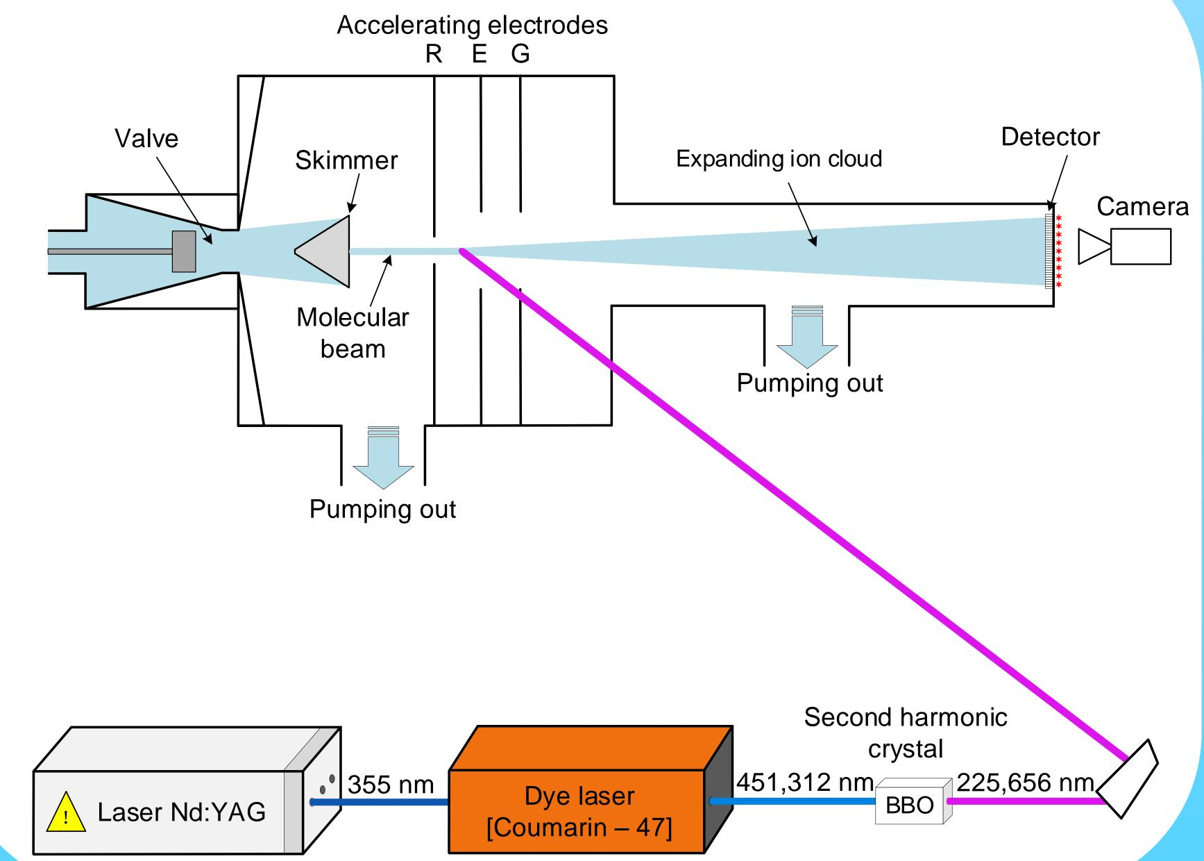
Energy of Xe -  $O_2$  complex  $D_{vdW}(Xe - O_2) = 2T_0 - 2T_1(1 + (\frac{2}{3}(\beta + 1)\frac{m_0}{m_{Xe}}))$  $T_0, T_1$  -kinetic energy of  $0^+$  formed from photodissociation of  $O_2$  and Xe –  $O_2$  respectively,  $\beta$  – anisotropy parameter
