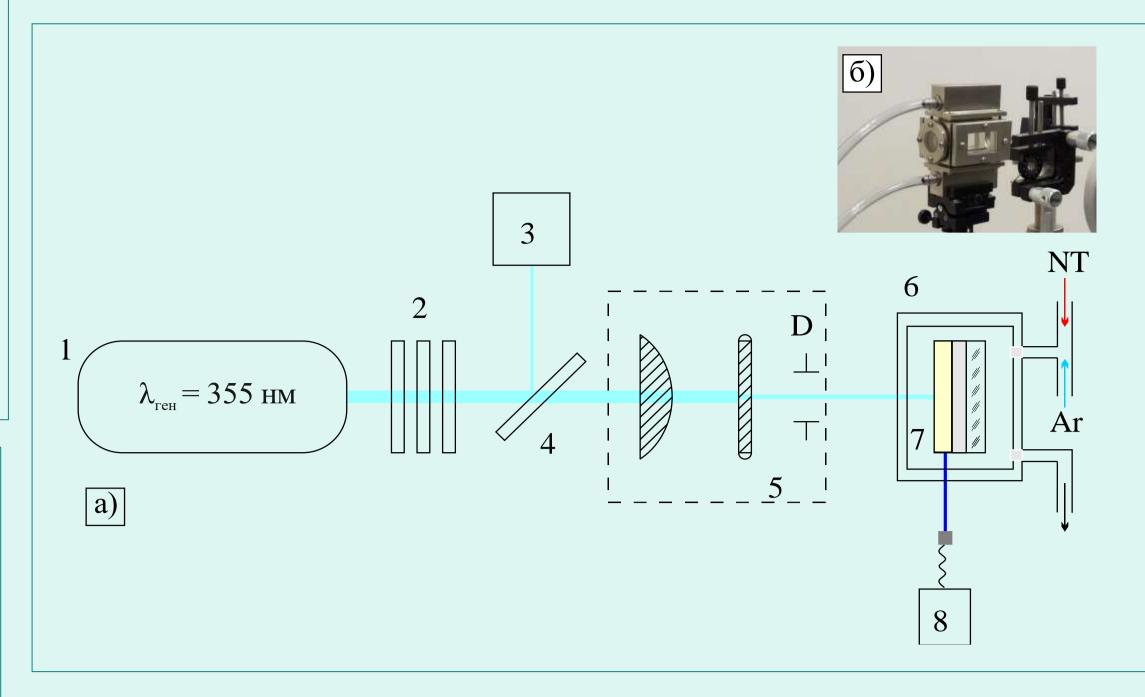
Fig. 3. (a) Scheme of the setup for measuring the spectraluminescent and lasing characteristics and (b) gas cell photograph: (1) Nd3+ : YAG laser (1 = 532 nm); (2)system of non-selective light filters; (3) Gentec EO ED-100A-UV energy meter; (4) beam splitter; (5) pump beamforming optical system; (6) gas cell; (7) thin-film sample under study;( 8) AvaSpec-2048 spectrometer; (b) photo of sealed cuvette.
