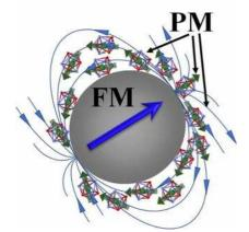
Fig. 1. Model of a composite material based on PrDyFeCoB microparticles (MP) and Er<sup>3+</sup> complex (PM). The internal field of particles is indicated by an arrow. The Er<sup>3+</sup> complex is located in the region of the stray field of microparticles.
